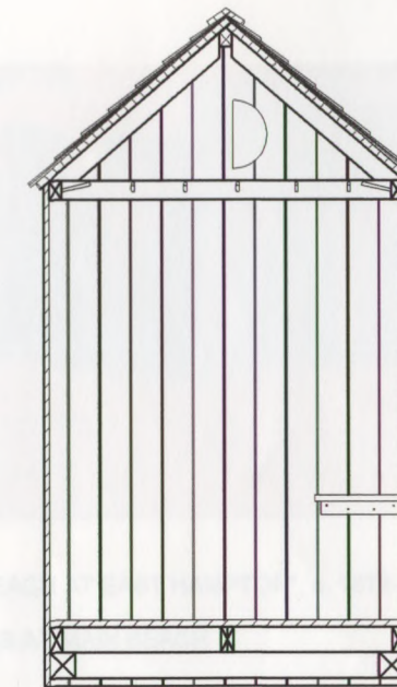
BUILDING SECTION LOOKING AT SOUTH INTERIOR WALL WITH BENCH RESTORED AND SHOWING PEGS FOR CLOTHING
